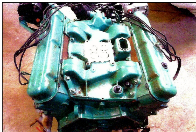
Notice how the intake manifold and carburetor base are located lower than usual, due to the engine having to be mounted higher than usual above the front drive transmission and axle.
